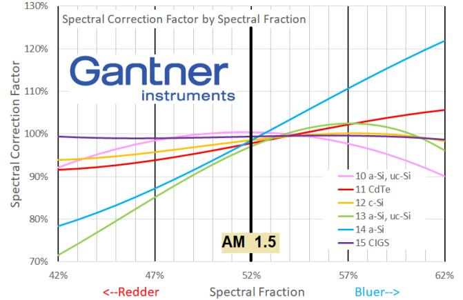
Fig. 7. Simplified spectral correction factor vs. spectral fraction from a smooth fit to measured GI OTF data.
