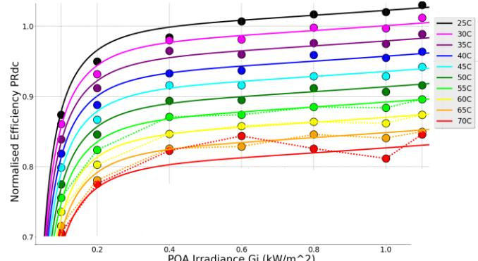
Fig. 13. MPM fit (smooth line) and linear interpolation (dotted) for a poor quality indoor matrix measurement of a cSi module,
