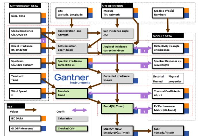
Fig. 2. Flowchart of process to generate an energy yield with data checks marked in purple
