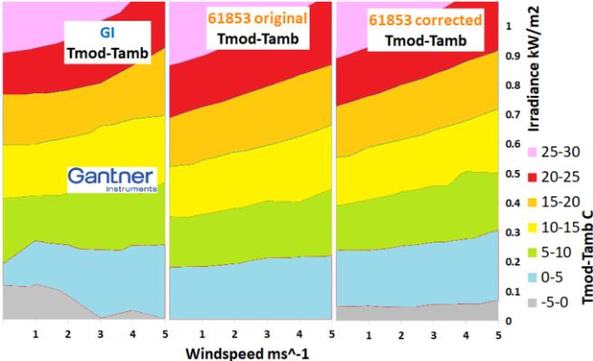
Fig. 9.  $T_{RISE}$  vs. Windspeed and measured Irradiance (left to right) measured (GI OTF), 61853 fitted (4) and 61853 corrected (5)
