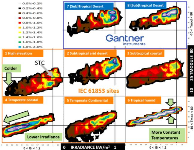
Fig. 3. Percentage of total yearly insolation (colours) per irradiance bin (0 to 1.2 kW/m<sup>2</sup> x-axis) and temperature bin (-10 to 80C y-axis) for different sites where #1-6 61853 vs. GI (top row) are #7 Tempe AZ and #8 Middle East.
