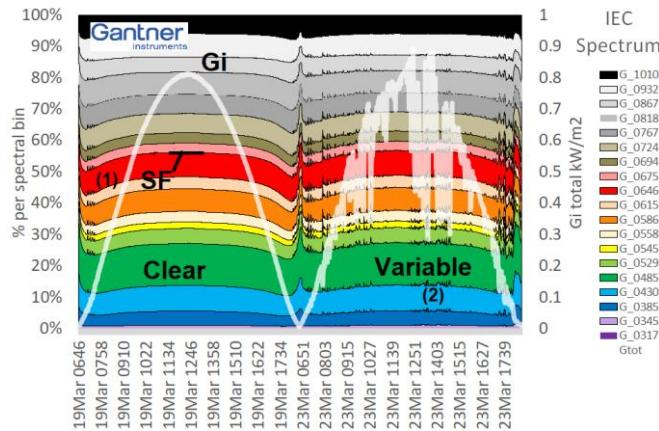
Fig. 6. Gantner Instruments’ measurements of spectrum bands as defined in 61853-3 for clear and variable days in Tempe, AZ.
