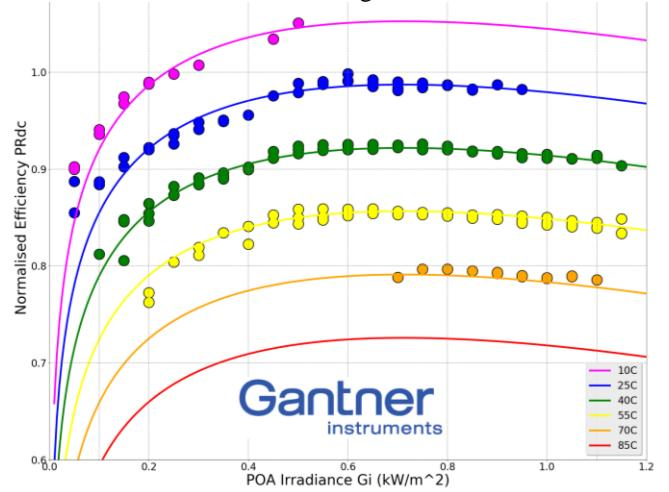
Fig. 11. GI OTF average matrix measurements (dots) for #12 c-Si module. Smooth lines show the fit from the MPM/LFM model with an rms error of ~0.5%
