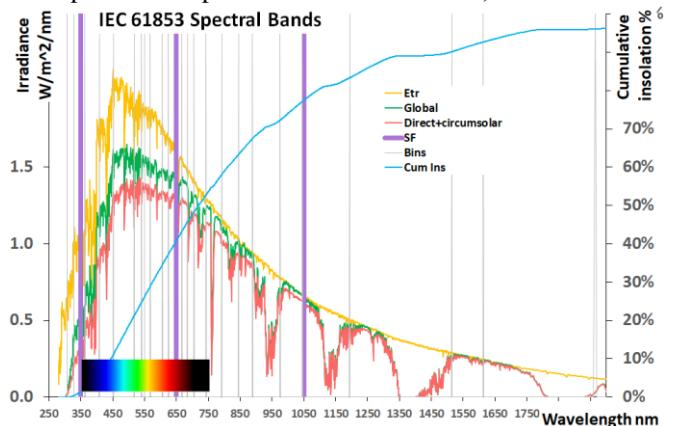
Fig. 5. IEC 61853-3 spectral bin widths vs. ASTM G173-03 spectra and SF limits of 350,650 and 1050nm [8].
