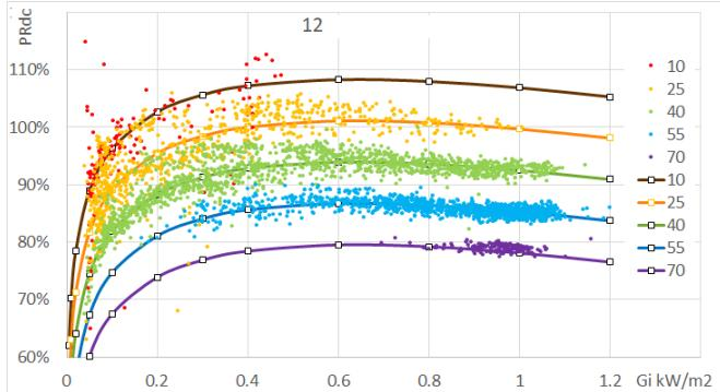
Fig. 12. GI temperature corrected outdoor raw measurements (dots) for a cSi module, fitted with MPM
