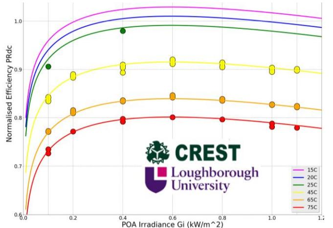
Fig. 10. CREST [10] indoor matrix measurements (dots) for a typical c-Si module. Smooth lines show the fit from the MPM/LFM model with an rms error of 0.23%
