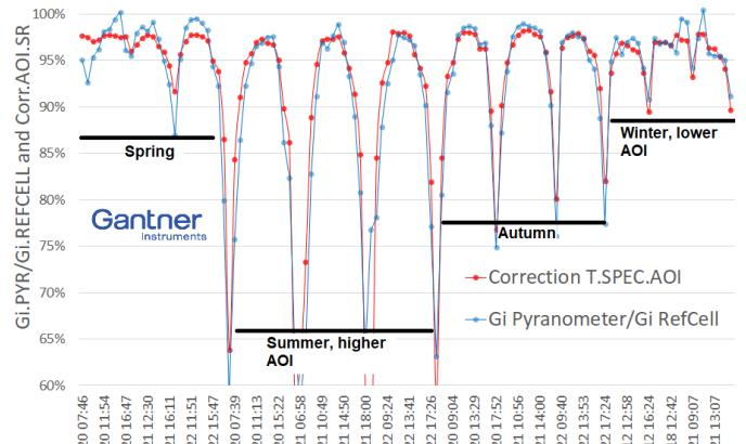
Fig. 8. Spectral and Angle of incidence correction to a Silicon reference cell compared with a pyranometer.
